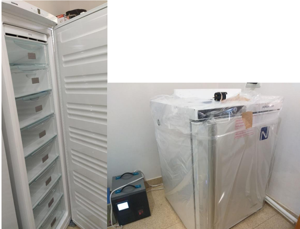
Figure 13: -20 °C (left) and -80°C (right) freezers now at the National Seed Bank of Armenia. Although many orchids are able to be stored in -20°C, others lose viability quickly, and may require ultracool conditions (e.g. -80°C).
